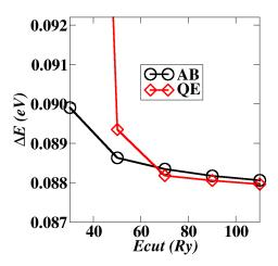
Fig. Plot of the energy difference between optimized structures of  $Na_4P_2S_6$  in the hexagonal  $P\bar{3}1m$  (#162 in the International Table of Crystallography) relative to the centered monoclinic structure C2/m (#12) as a function of the kinetic energy cutoff energy used in the calculation. Results are given in units of eV/Formula Unit and calculations were performed with the ABINIT (AB) and the QUANTUM ESPRESSO (QE) codes using the PBESOL functional.
