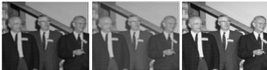
FIGURE 1.3 Restoring Gaussian blur with zero boundary (left), periodic boundary (middle) and Neumann boundary (right) conditions.
