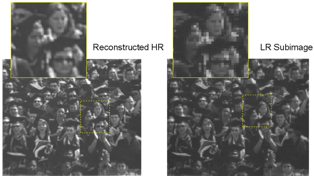
Figure 4. Digital super resolution reconstruction (shown on the left) of low resolution multi-aperture images captured with the PERIODIC camera. For this example 16 low-resolution subimages were used for the reconstruction. The measured resolution improvement was approximately 3X.
