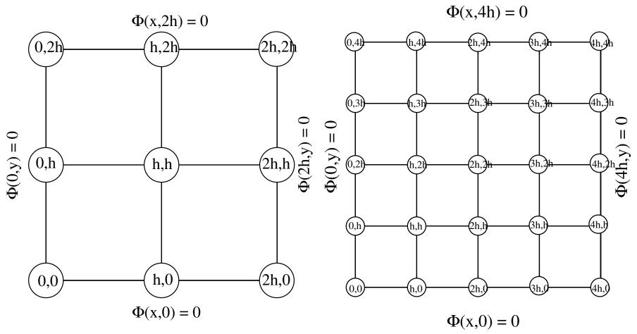
$3 \times 3$  grid for solution of the Poisson equation within a 2-dimensional square.
