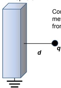
Consider a grounded metal sheet, a distance  $d$  from a point charge  $q$ .
