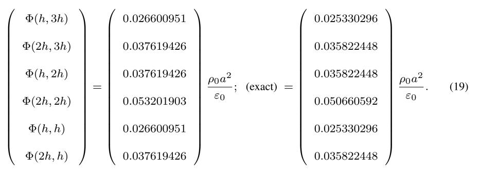
We see that the results obtained with a smaller mesh has is much closer to the exact results than those for the larger mesh.
