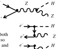
The three diagrams are sketched at right. The two new ones both have the Higgs coupled to an electron, but since the electron mass is so tiny compared to the Z mass, it will be pretty negligible. If we let p and p' be the momenta of the initial electron and positron respectively, then the amplitude for the process (considering only the first diagram) will be given by
