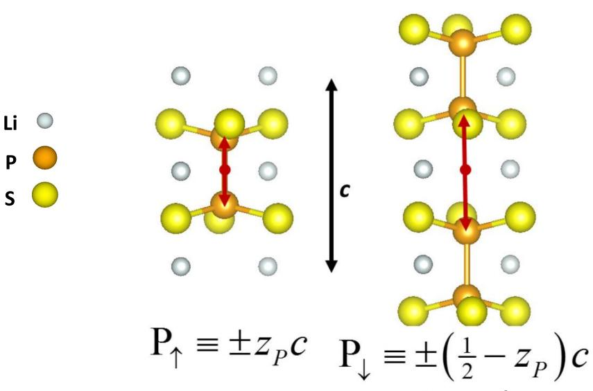
Structural variation can be mapped on to a two-dimensional hexagonal lattice with each P configuration taking P or P √ settings; Li and S configurations fixed
