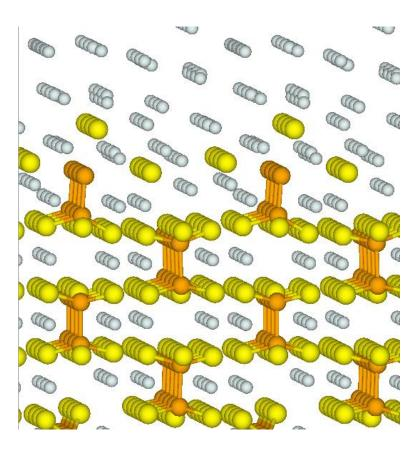
Reactivity of Li/Li<sub>4</sub>P<sub>2</sub>S<sub>6</sub> interface models consistent with experimental observation that Li/Li<sub>4</sub>P<sub>2</sub>S<sub>6</sub> /Li cells could not be cycled
