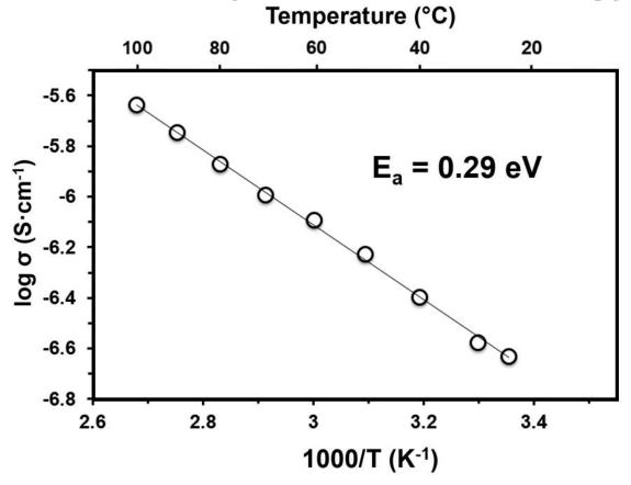
$2.38 \times 10^{-7} \text{ S/cm}$  at  $25^{\circ}\text{C}$  and  $2.33 \times 10^{-6} \text{ S/cm}$  at  $100^{\circ}\text{C}$   $\text{Li}_4\text{P}_2\text{S}_6$  pressed pellets with blocking (Al/C) electrodes
