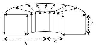
magnetic flux density  $\mathbf{B}(\mathbf{x}) = B(\rho, z)\hat{\mathbf{\phi}}$  in cylindrical coordinates. Find  $\mathbf{B}$  at all points inside or outside the tokamak, and find the total magnetic energy stored inside the tokamak.
